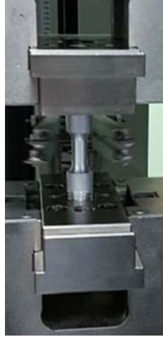
Fig. 1 The sample subjected to the cyclic tension–compression test
