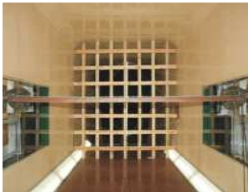
Fig. 3: IRR bridge model and grids to generate turbulent flow in wind tunnel
