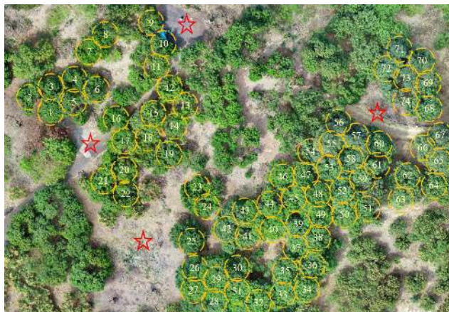
FIGURE 9. Locations where pesticide treatments are needed. The yellow-dashed circles represent the agricultural drone's range for spraying pesticides; the red stars are the positioning points for calibration before each drone flight.
