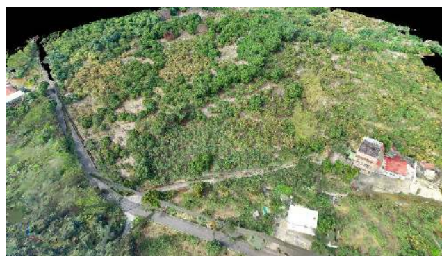
FIGURE 7. DSM data with a resolution of 1.42cm/pixel generated from the aerial images acquired by the UAV.
