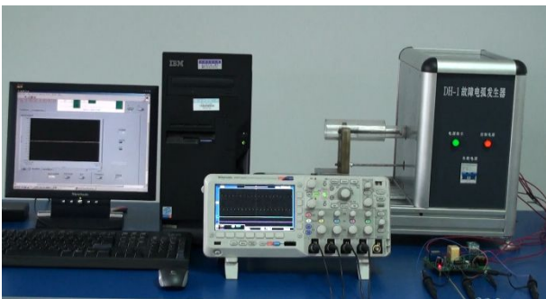
Fig. 2. Experiment setup for series arc faults generation and data acquisition with computer and oscilloscope.
