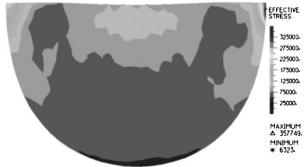
3 Distribution of effective stress computed 10 on outer surface of open leaflet
