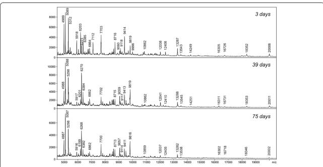
**Figure 5 Effect of the storage conditions on the spectra quality.** Comparison of MALDI-TOF MS spectra of *Phlebotomus tobbi* females stored in 70% ethanol for 3, 39 and 75 days.
