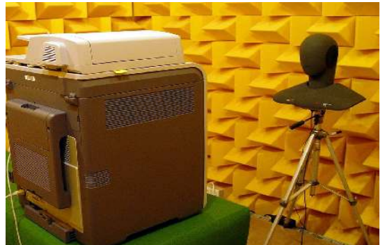
Fig. 2 Printing sound recording through HMS III artificial head
