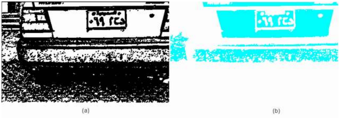
Figure 6-10: (a) Vector Angle based edge map of image shown in Fig 6-4(b). (b) 8-connected areas of the image shown in (a).
