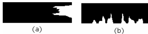
Figure 6-15: Horizontal (a) and Vertical (b) projection profile of the plate based on the selected cluster (cluster 2) from the image shown in Fig 6.14.
