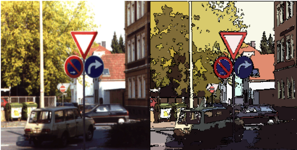
Figure 2-2: Example of a CSC-segmented scene, where all found objects (trees in the CSC data structure) are presented by the outer border and the involved pixels in the mean color of the object. [72]
