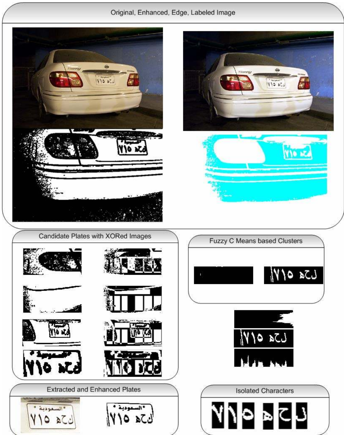
Figure 7-5: Image taken under low light. The plate's background color is similar to the foreground (VA implementation)
