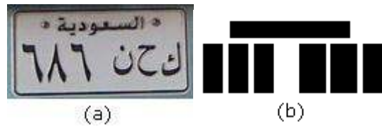
Figure 6-8: (a) Standard Saudi Arabian License Plate. (b) Saudi Arabian License Plate Template ( I_T )
