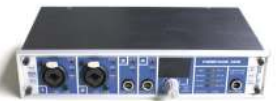
RME Fireface 400 external sound card. The display was covered with black tape to not distract observers.
