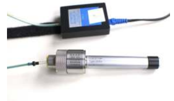
A G.R.A.S. RA0045 in-ear headphone coupler connected to a B&K Falcon 2669 microphone preamplifier (bottom) is coupled to an Etymotic headphone (top, bottom left).
