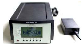
A B&K Nexus 2690 conditioning amplifier with power supply.
