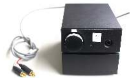
NAIM headphone amplifier (top) with external power supply (bottom) and RCA signal input plugs.
