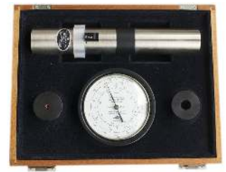
A Brüel & Kjær 4220 pistonphone (top) including a barometer (bottom) to correct for deviations in sound level and standard frequency due to the ambient air pressure.
