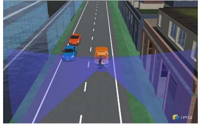
Fig. 5: Collision detected in simulation at parameter values subject vehicle velocity = 58.06km/hr, pedestrian speed = 17.82km/hr, Crossing angle = 4.57°, deceleration rate = 3m/s 2 . This test case gives a function value of -5
