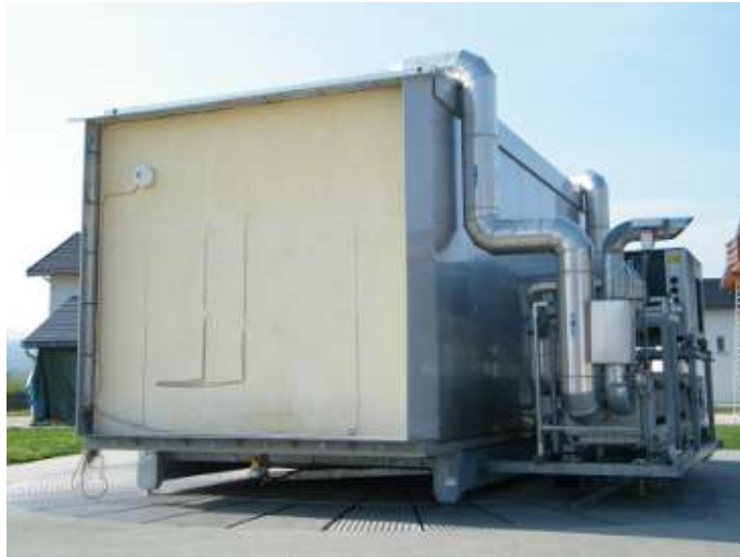
Figure 5: PASSSYS instrumented test cell
