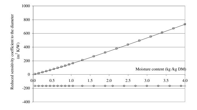
Figure 8 – Reduced sensitivity coefficients of the contact resistance to the stirrer speed and the moisture content for  $10^{-3}$  m activated alumina balls.
