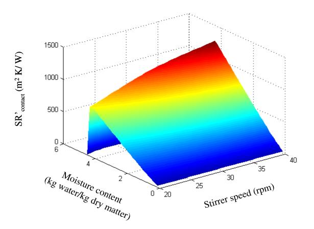
Figure 9 – Reduced sensitivity coefficients of the penetration resistance to the stirrer speed and the moisture content for  $10^{-3}$  m activated alumina balls.
