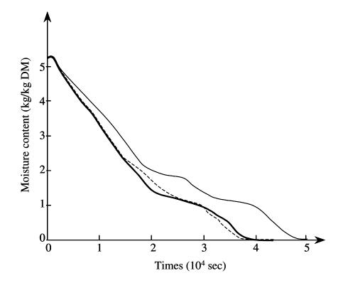
Figure 16 Measured (dot) and adjusted (line) drying kinetics of an anaerobically digested sludge ( (+), d=1.15  $10^{-3}$  m) and an extended aeration one (<sub>O</sub>), d=0.9  $10^{-3}$  m) for T<sub>wall</sub> = 160°C and  $\omega$  = 40 rpm.
