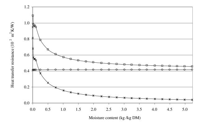
Figure 14 – Measured (dot) and adjusted (line) drying kinetics of the digested sewage sludge coming from Albi City for ( $\Box$ ) T<sub>wall</sub> = 160°C and ( $\circ$ ) T<sub>wall</sub> = 120°C ( $\omega$  = 40 rpm, d=1.15 10<sup>-3</sup>m).
