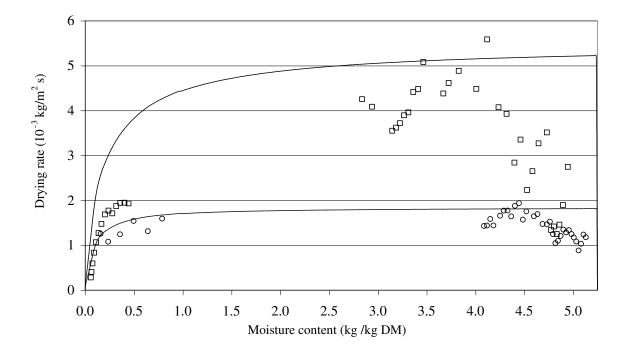
Figure 15 – Influence of the stirrer speed, (+)  $\omega = 20$  rpm, (o)  $\omega = 40$  rpm and (--) $\omega = 60$  rpm, on the experimental drying kinetic (T<sub>wall</sub> = 120°C).
