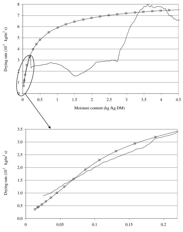
Figure 11 – Measured( —) and adjusted ( —) drying kinetics of the digested sewage sludge coming from Albi City ( $T_{wall} = 180^{\circ}$ C,  $\omega = 40$  rpm, d=1.15  $10^{-3}$ m).
