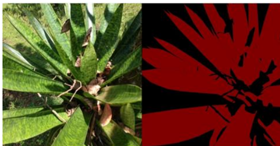
Figure 2. Aerial image (left) of W. kupperiana and the annotated image (right) with the mask (red) containing pixels of the target plant. Dried parts of the plants were not included in the masks.
