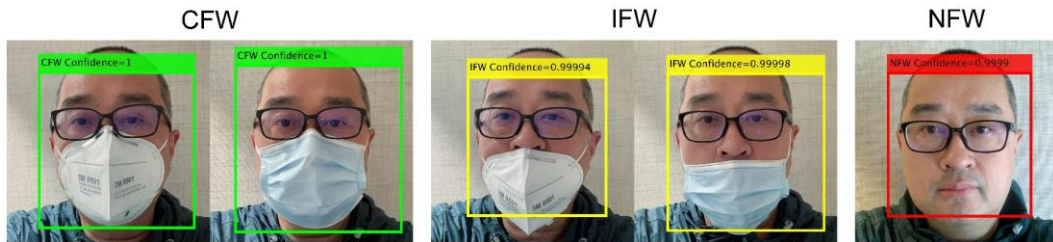
Figure 4. Identification Examples. The labels showed the identification results and confidences of SRCNet. CFW = correct facemask-wearing (green), IFW = incorrect facemask-wearing (yellow), NFW = no facemask-wearing (red).
