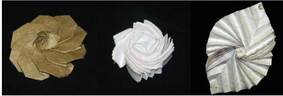
Figure 1. Example of an origami structure (left) and flasher hat mechanism in its fabricated (middle) and deployed form (right).
