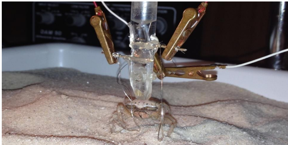
Figure 4: Experimental setup with animal suspended over sand-filled arena
