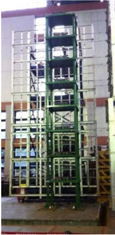
Fig. 7. A photo for an eight-storey steel frame under shaking table tests.
