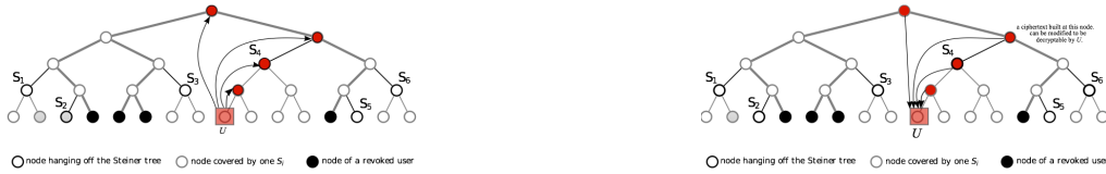
Fig. 1. Comparison between Asano’s method and our method. In Asano’s method, from a private key, a user U can derive keys at any nodes on the path from its leaf to the root. Our method can be seen as a dual of Asano’s method where a ciphertext at a node can be modified to be decryptable with keys at lower nodes.
