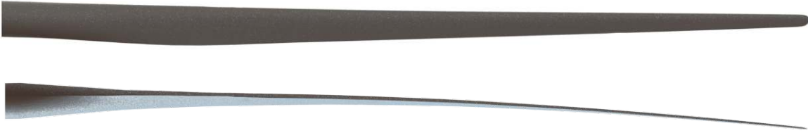
Figure 2-1. View from the suction side (top) and trailing edge (bottom) of the offshore wind turbine blade
