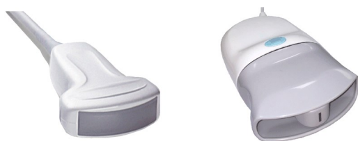
Figure 1: Comparison of the SonoSite Multichannel Array Transducer (left) [9] and the Prototype Single Element Ultrasound Scanner (right)
