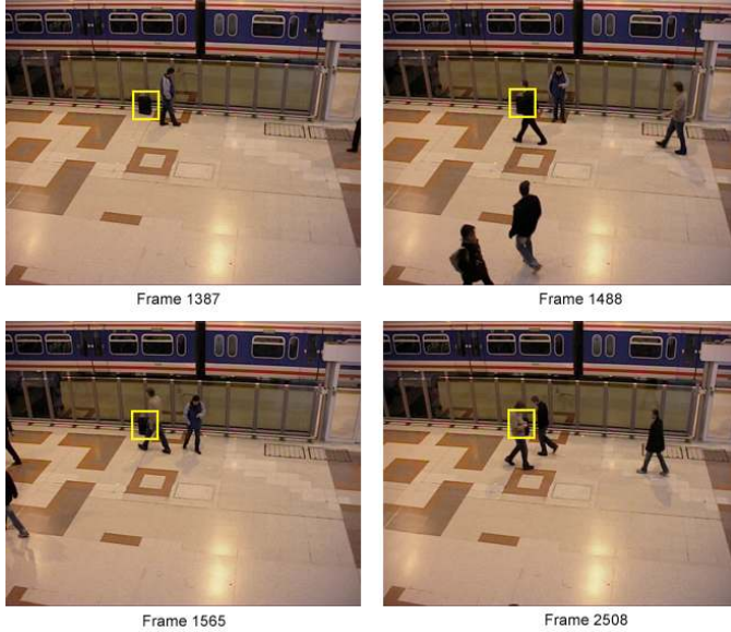
Fig. 2 Video sequence from the PETS 2006 dataset used to compare results from the adaptive edge orientation based technique with cross-correlation as used in Tian et al. [3]. The tracked object is occluded in Frame 1488, 1565 and 2508.
