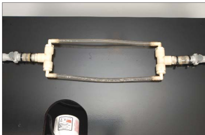
Fig. 3. To illustrate concepts of current conservation in circuits involving resistors in parallel, the light bulb tubing is replaced by two small Tygon tubes. Photo by Pierce Bounds
