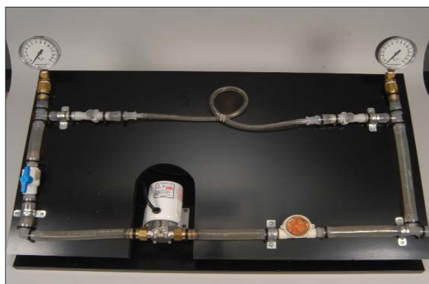
Fig. 1. Photograph of the Glitter Electric Circuit Analog (GECA) showing the pump (battery), the valve (switch), the thin tube (light bulb), a flow meter (ammeter), and two pressure sensors that indicate the pressure difference across the thin tube. Not shown is the valve that shuts off the filler/drain tube at the bottom right of the circuit. Photo by Pierce Bounds
