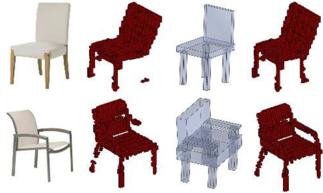
Figure 9: Part symmetry induced volume refinement. Given a 2D image, a volumetric shape is recovered using 3D-GAN [22] where the missing voxels break the symmetry of the object. Our recovered 3D structure helps complete the volume based on part symmetry relation.
