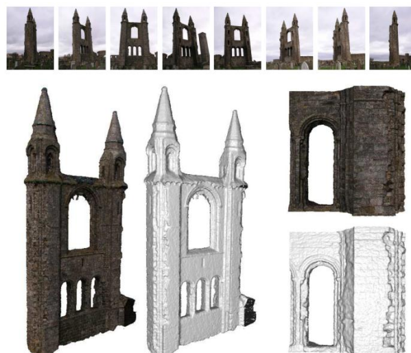
Figure 1: Church ruin St. Andrews, Scotland. 43 images with 5 Megapixels acquired in a circle around the object. Left: point cloud from dense image matching, right: meshed surface derived by volumetric range integration.
