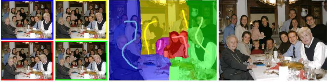
Figure 23: From a set of five source images (of which four are shown on the left), Photomontage quickly creates a composite family portrait in which everyone is smiling and looking at the camera (right). Users simply flip through the stack and coarsely draw strokes using the designated source image objective over the people they wish to add to the composite. The user-applied strokes and computed regions are color-coded by the borders of the source images on the left (middle). (Copied, with permission, from (Agarwala et al. 2004)).
