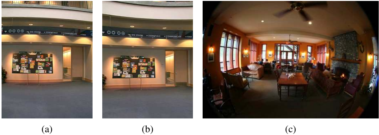
Figure 9: Examples of radial lens distortion: (a) barrel, (b) pincushion, and (c) fisheye. The fisheye image spans almost a complete 180° from side-to-side.
