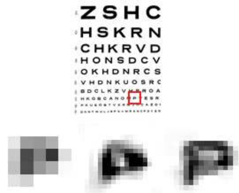
Fig. 7: Image with repetitions. Top images shows the input bottom images show: (left) input pixels, (middle) output produced by our method, and (right) the results of Glasner et al. [2009].
