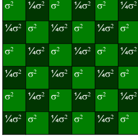
Figure 2. When demosaicing is performed with linear interpolation, the interpolated green pixels have lower variance than the original green pixels. Assuming pixel values from green photosites in the Bayer array are IID with variance \sigma^2 , this image represents the variance from which each pixel value is drawn. The spatial pattern of variances is the basis for detecting the presence of demosaicing.
