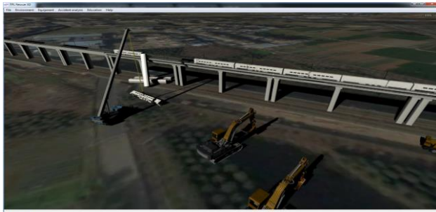
Figure 6. Simulation of lifting derailed trains
