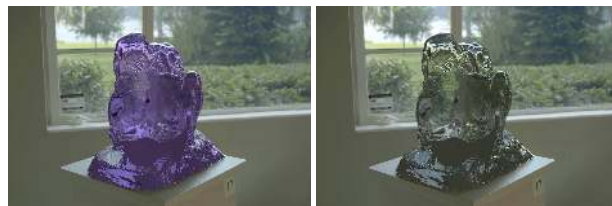
Figure 17: Colored glass (left) and darkened glass (right) simulated with a linear attenuation to achieve color ( G in 23), and non-linear scaling to simulate dark glass (24). The refractions in these images are different from the ones shown in Figure 16 due to a different choice of filter kernel sizes of the bilateral filter, as well as a different choice of scale factor s .
