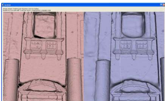
Figure 14: San Nicola 136 dataset – on the left High Resolution photos 3D model, on the right Low Resolution photos 3D model
