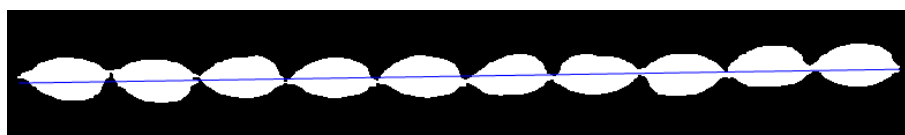
Figure 6. Binary image of rice grains without overlap and its main axis.
