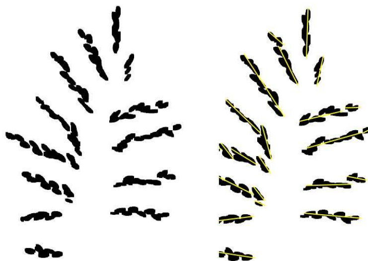
Figure 4. Main axis of each connected region.
