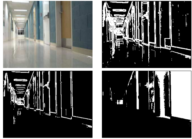
Fig. 3. TOP-LEFT: A typical corridor image. TOP-RIGHT: Pixels with gradient magnitude greater than a threshold are shown in white. BOTTOM-LEFT: Using the separating curve from Fig. 5, the edge pixels mostly follow the boundaries of the wall, door frames, and floor. BOTTOM-RIGHT: The original image thresholded by a value determined by the separating curve, thus revealing the structure of the corridor.
