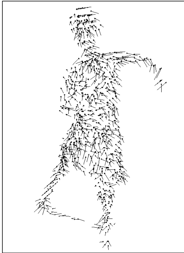
Figure 3.5: The recovered scene flow shown as a 3-D needlemap. The flow recovered is dense, so every surface voxel on the shapes shown in Figure 3.5 has a flow vector. In this view, the flow is shown for all voxels (including ones on hidden surfaces).
