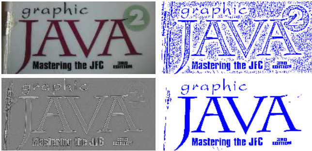
Fig. 2. The steps of the proposed binarization method. (Top-left - input image, top-right - local binarization for dark text on light background (the candidate text regions are shown in blue), bottom-left - the seeds resulting from incorporating local binarization and the Laplacian of the image intensity, bottom-right - the binarization after global optimization for dark text on light background. The candidate text regions are shown in blue.
