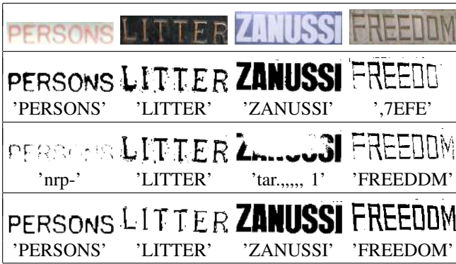
Fig. 1. A comparison of cropped image binarization results of methods with top OCR accuracy (labels flipped where appropriate). From top to bottom line: (1) original image, (2) Niblack, (3) Non-linear Niblack, (4) Proposed.
