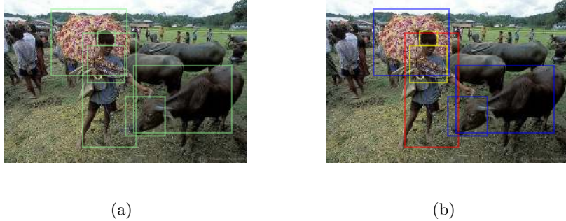
Fig. 3: (a) Image with detected regions; (b) An example of query region in the image (man in the red bounding box), and its neighbor regions (regions in blue bounding boxes, bull, umbrella, etc), child regions (regions in the yellow bounding boxes, hair, cloth).
