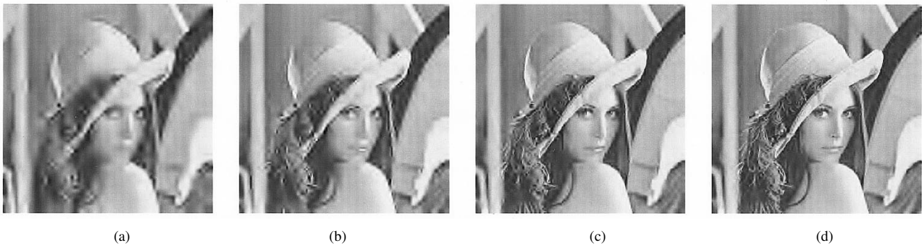
Fig. 12. Illustration of where bits go. Sequence of reconstructions at very low bit rates: (a) 512 bytes, (b) 1024 bytes, (c) 2048 bytes, (d) 3072 bytes; recall that the original has 262 144 bytes. Observe how textured regions receive a significant amount of bits.
