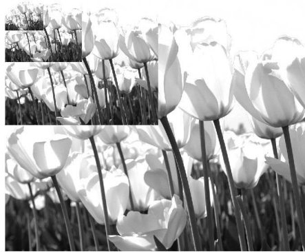
Fig 5. Generation of Gaussian pyramid with a reduction factor 2
