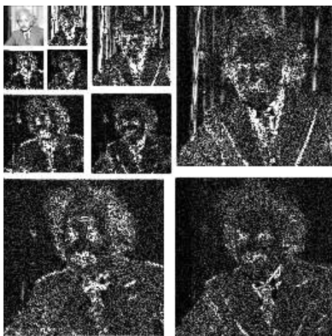
Figure 4: Coefficient magnitudes of a wavelet decomposition. Shown are absolute values of subband coefficients at three scales, and three orientations of a separable wavelet decomposition of the Einstein image. Also shown is the lowpass residual subband (upper left). Note that high-magnitude coefficients of the subbands tend to be located in the same (relative) spatial positions.
