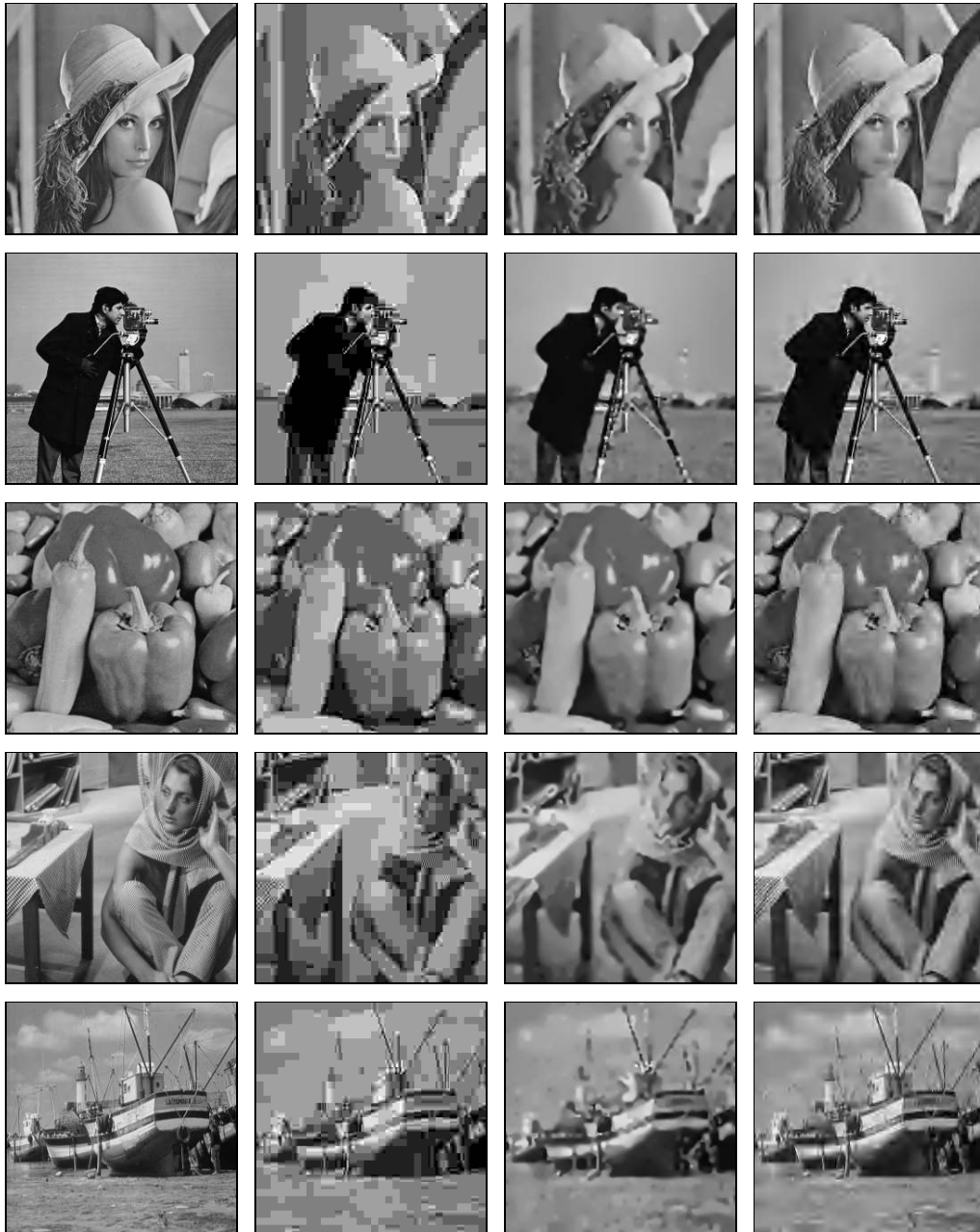
Figure 9: Comparison of compression methods at 0.2 bpp for different test images (rescaled to 257 \times 257 pixels). Rows, top to bottom: lena , cameraman , peppers , barbara , boats . Columns, left to right: Original image, reconstructed images after compression by JPEG, by EEDC, and by JPEG2000.
