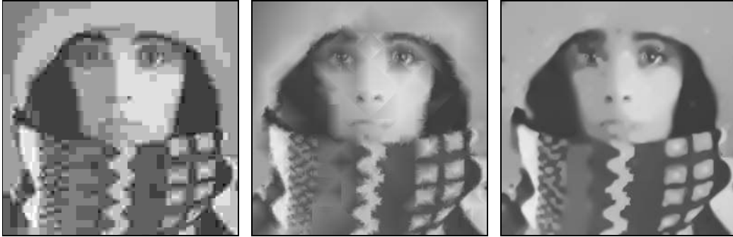
Figure 5: Comparison at high compression rates (0.2 bpp) for the test image trui . Left: JPEG. Middle: Q64+BTTC(L)-L. Right: Q64+BTTC(L)-EED.
