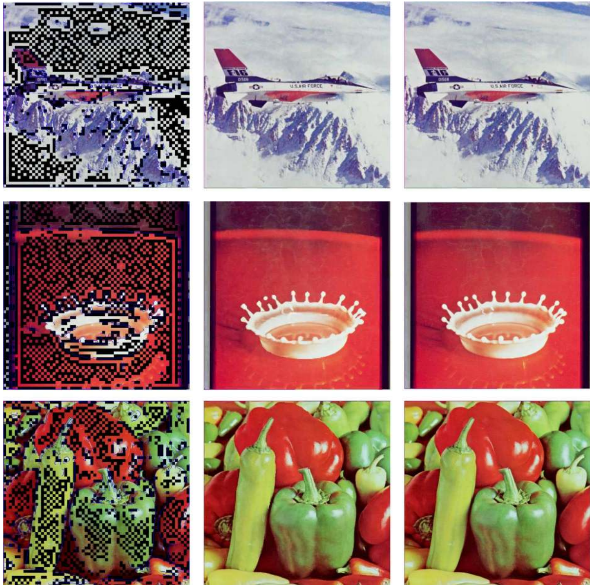
Fig. 9. Comparisons with baseline JPEG on test images Jet, Milk, and Peppers. From left to right: removed blocks (black blocks) and assistant edge information (blue curves); reconstructed image by our scheme; reconstructed image by baseline JPEG.
