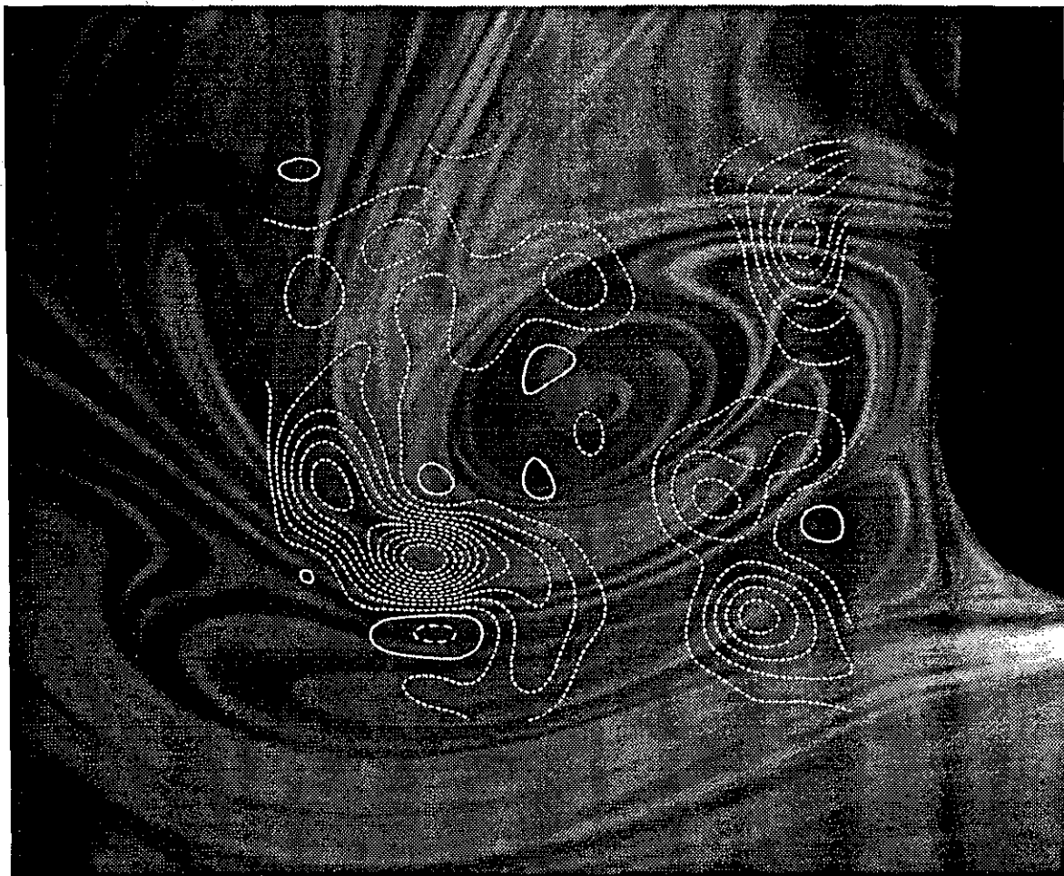
FIG. 14 Contours of constant second invariant of the rate-of-strain tensor (Eq. 45), q_s = -\frac{1}{2} \left[ \left( \frac{\partial u}{\partial x} \right)^2 + \left( \frac{\partial v}{\partial y} \right)^2 - \frac{1}{2} \left( \frac{\partial u}{\partial y} + \frac{\partial v}{\partial x} \right)^2 \right] . Contours spaced by 0.5 \text{ s}^{-2} .
