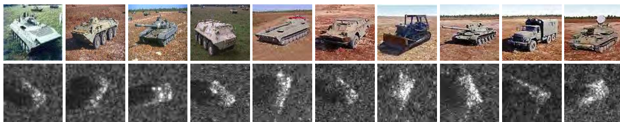
FIGURE 7. Optical images (top) and SAR images (bottom) of ten kinds of target samples. According to the order: BMP2, BTR70, T72, BTR60, 2S1, BRDM2, D7, T62, ZIL131, and ZSU23/4.
