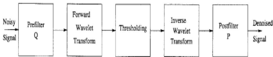
Figure2: Diagram of wavelet based image De-noising
