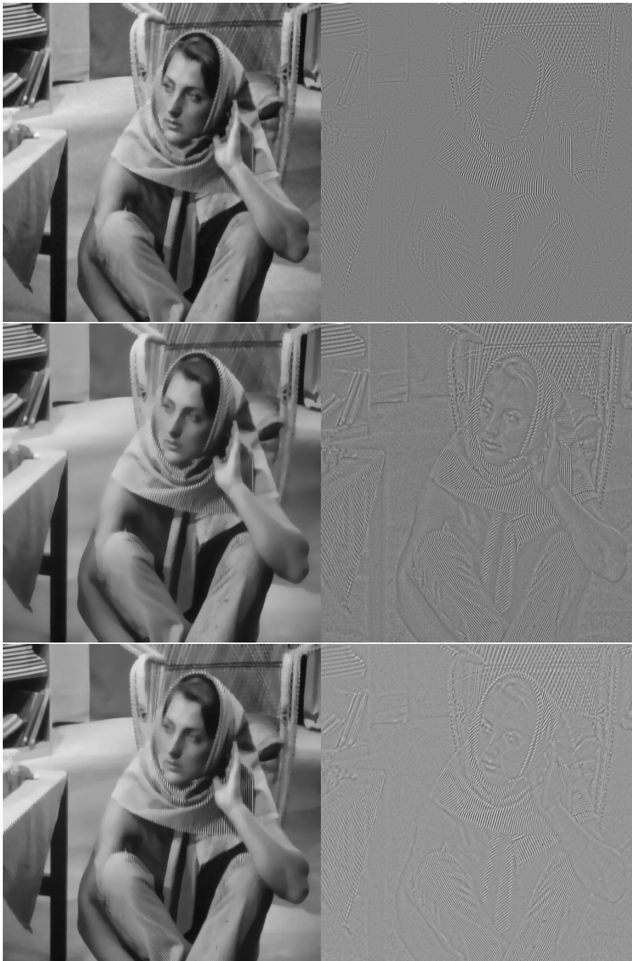
FIG. 6. u (left) and v (right) using the new method (top), the TV model (middle), and [21] (bottom). We choose \lambda in the TV model such that the L^2 -norm of v is the same in the first and second rows.
