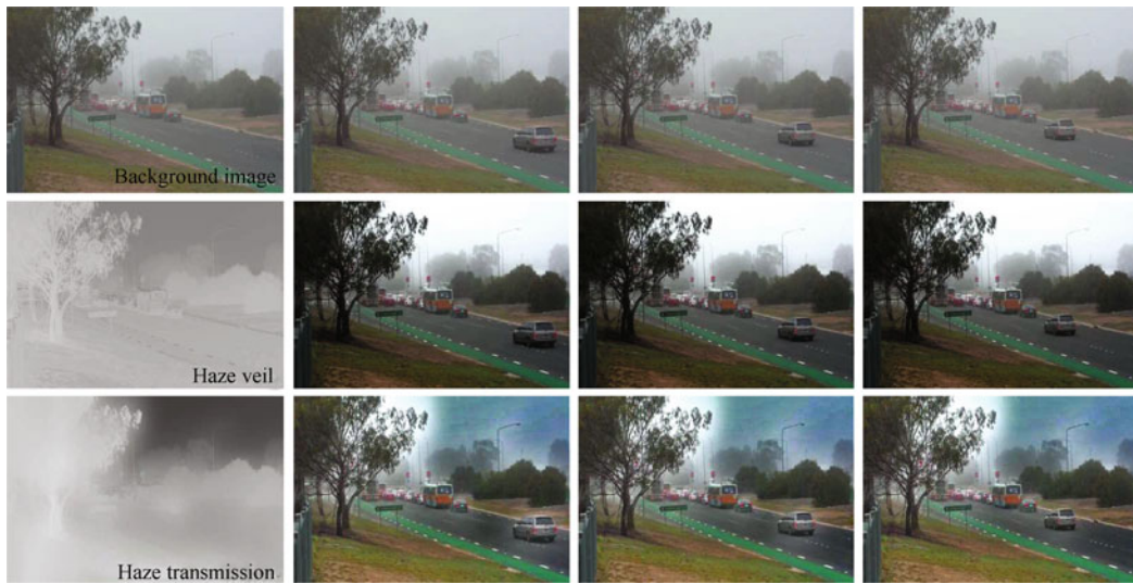
Fig. 6 Our video result. First row: estimated background image and three original frames from video. Second row: universal haze veil and the enhanced frames obtained by using the same veil. Third row: universal haze transmission and the restored frames obtained by using the same transmission
