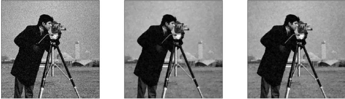
Figure 7. From left to right: (a) the cameraman image degraded by white noise with standard deviation \sigma = 15 ; (b) denoising of the previous image by the filter defined by Eq. (5) with parameter values p = 0.2 and \varepsilon = 10^{-2} ; (c) denoising by the same filter with parameter values p = 0.1 and \varepsilon = 10^{-2} .
