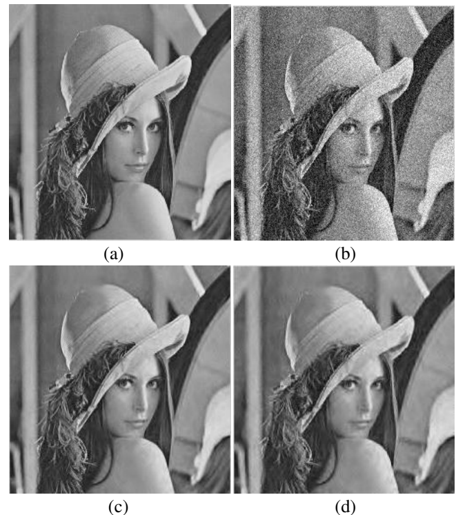
Fig.- 13: (a) Clean Lena Image (b) Noisy image at \sigma = 20 (c) Denoised image at \sigma = 20 (d) Denoised image at \sigma = 30
