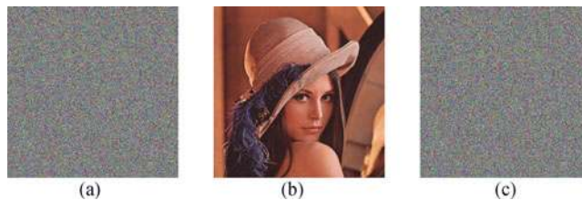
Fig. 7. Decryption key sensitivity analysis: (a) Encrypted image: key = 1234567890 123456. (b) Decrypted image: key = 1234567890123456. (c) Decrypted image: key = 1234567890123457.
