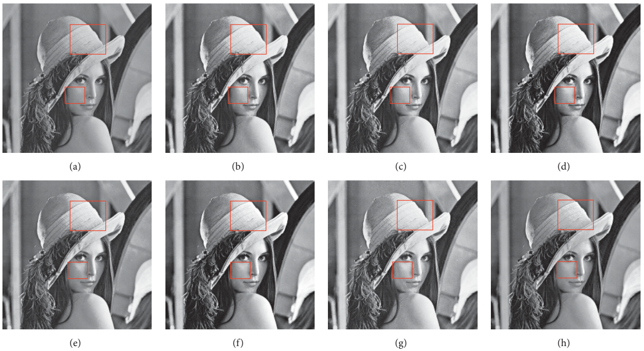
FIGURE 6: Results for Lena. (a) Original image. (b) DSIHE. (c) RMSHE. (d) MMBEBHE. (e) RSIHE. (f) ESIHE. (g) BHEBHD. (h) Proposed MVSIEH.
