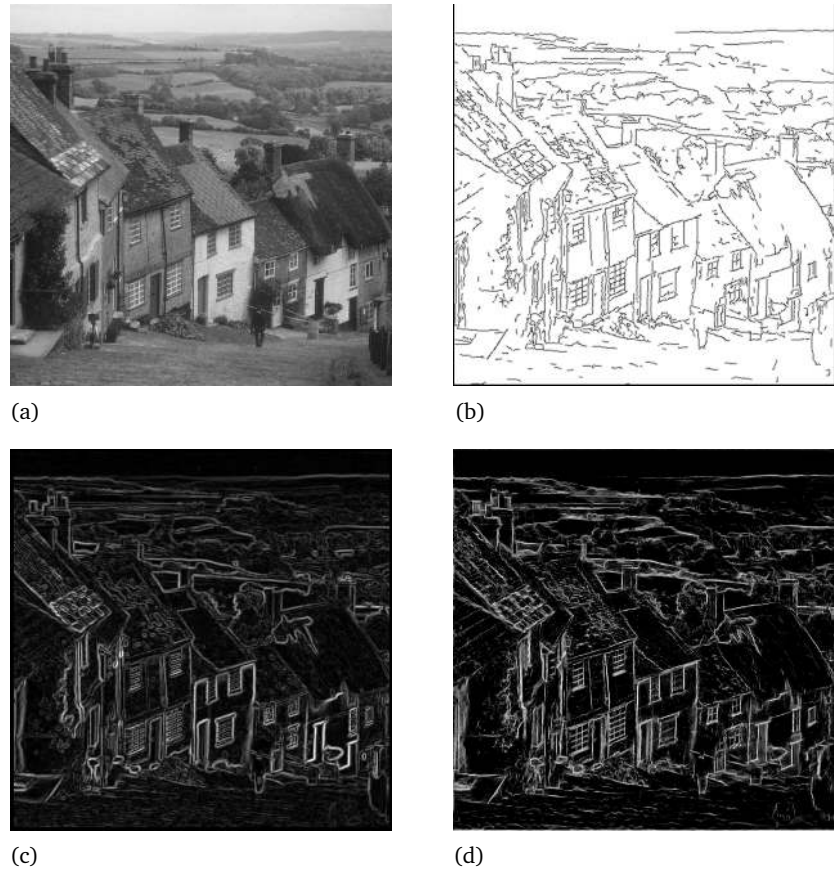
Figure 13. Goldhill image. This image illustrates the ability of the PC_2 measure to pick out fine features. The window panes and roof tiles in the nearer houses are clearly marked. (a) original image; (b) phase congruency feature map; (c) Canny edge strength image; (d) raw phase congruency image.
